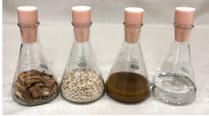
(From left to right) Wood chips, pulp, fermentation culture liquid, "MORISORA" bioethanol
